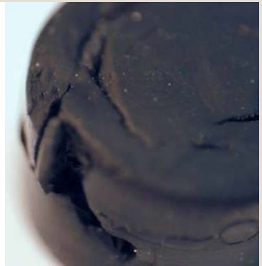
A damaged and deformed probe tip
